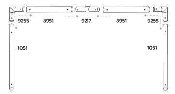
Fit the crossbar (step 4) to the base (step 3), affixing the 2 x 1051 to the 2 x 9255.
