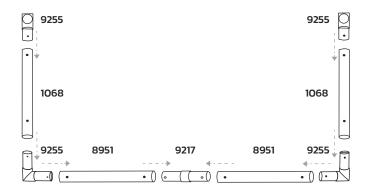
Assemble the crossbar and the upright section, attaching 8951 & 1051 to connectors.
